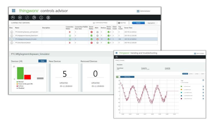
Description: See the state of all OPC Server installs in a single webpage. Dive deeper into device connectivity trending real-time data from PLCs.
